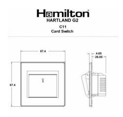
**Additional Notes** Adjustable Time Delay 10 seconds - 5 minutes. Suitable for 44mm and 54mm width Hotel Key Cards
