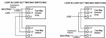
Note: When switching from more than position a two way dimmer can only be used in conjunction with switches i.e. Only one dimmer per circuit
